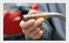
/ Radically new cooling concept, right through to the gas nozzle of the torch. For cool, precise working, and longer endurance times of wearing parts.
