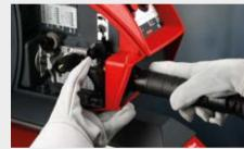
/ The Fronius System Connector serves as a central connection-point for all media. It lets users lock the hosepack simply and safely, with no tools, to ensure a guaranteed defined current transfer.
